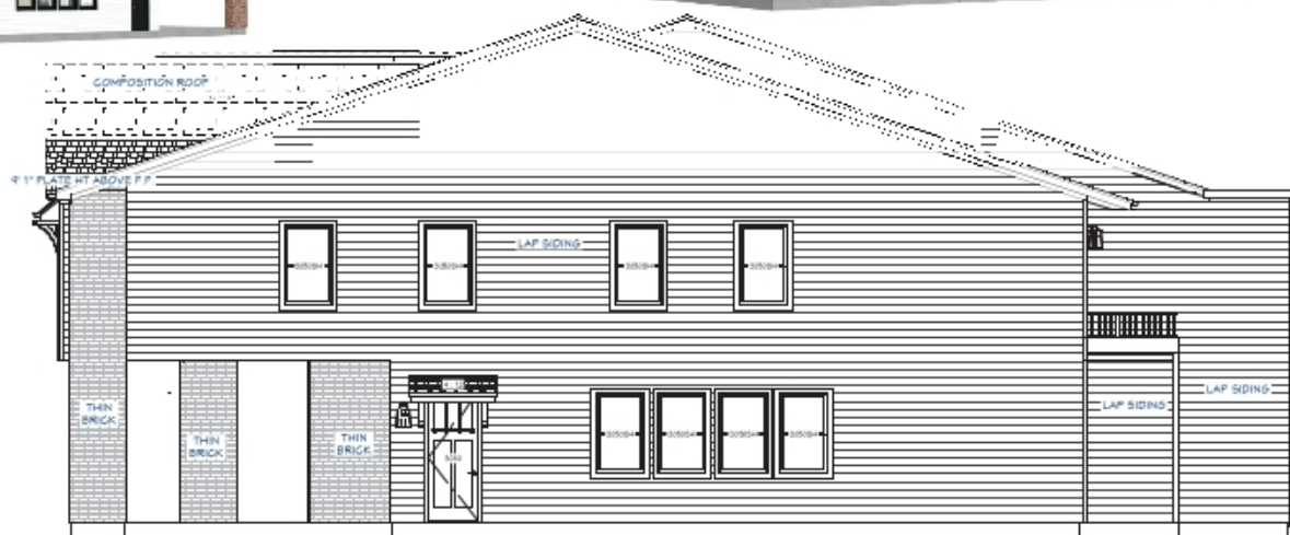
E4 EXTERIOR ELEVATION RIGHT 1/4 IN. = 1 FT
